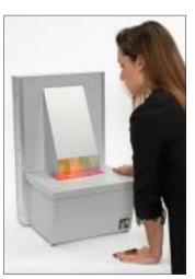
The SCV is uniquely designed to allow maximum light source selection so you can see your color under most commonly used light sources. Unit operates on 120V unless otherwise specified and uses common 24" fluorescent lamps.
